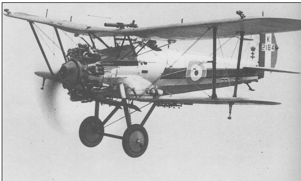
Bristol Bulldog K2184 of No.41 Squadron is seen here during a sortie from Northolt. Note the camera gun on the upper mainplane and the Squadron's 'crown & cross' motif on the fin.
