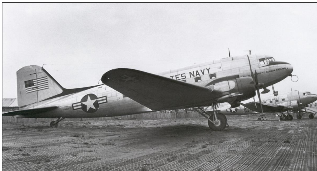
Douglas R4D, possibly of FASRON-76 is seen here at Hendon in 1951. The R4D was the naval equivalent of the United States Air Force's C-47 Skytrain. Note the pierced steel planking (PSP) that forms its dispersal at Hendon. (Les Vowels).
